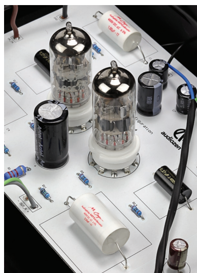
E88CC valves are employed for the pre-amp section. Audiozen sources new old stock (NOS) tubes for this.
